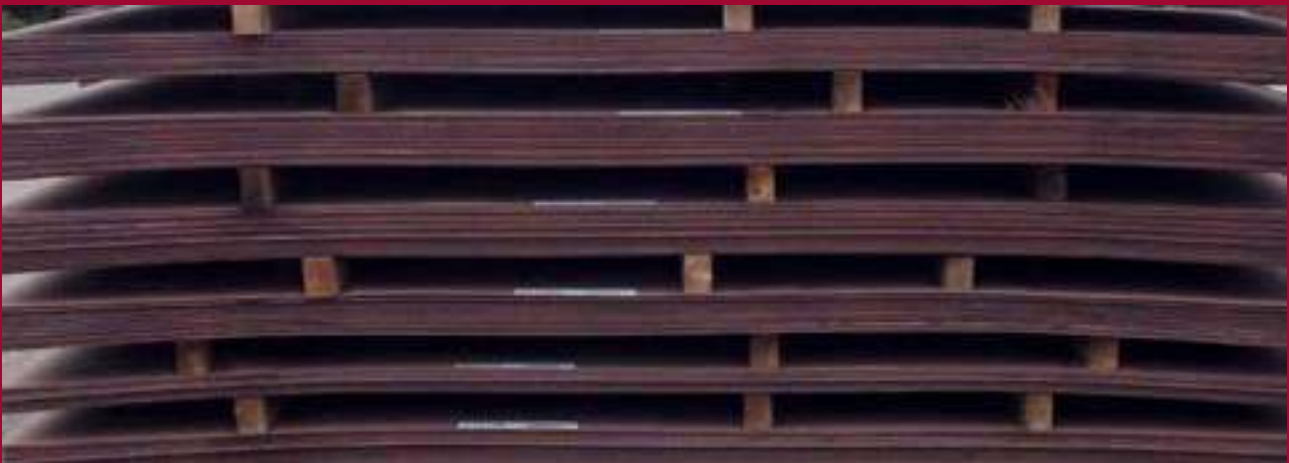
Figure 13b: Improperly stacked plates
