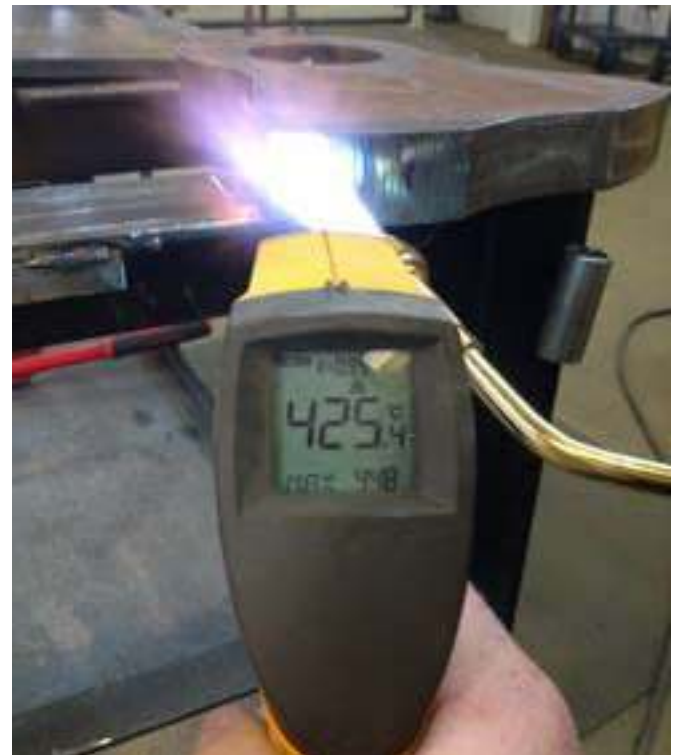
Figure 10: Temperature measurement during postheating.
