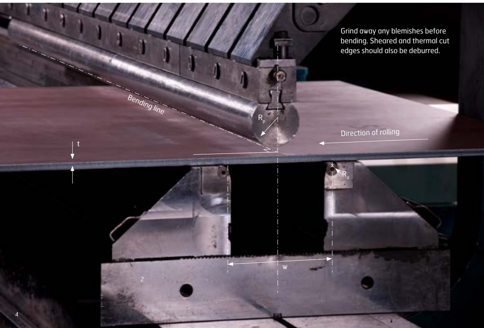
FIGURE 1 Bending transverse to the direction of rolling.
